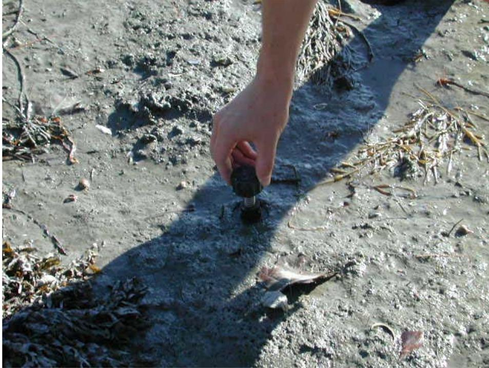
Figure 4. Measuring sediment shear strength.
