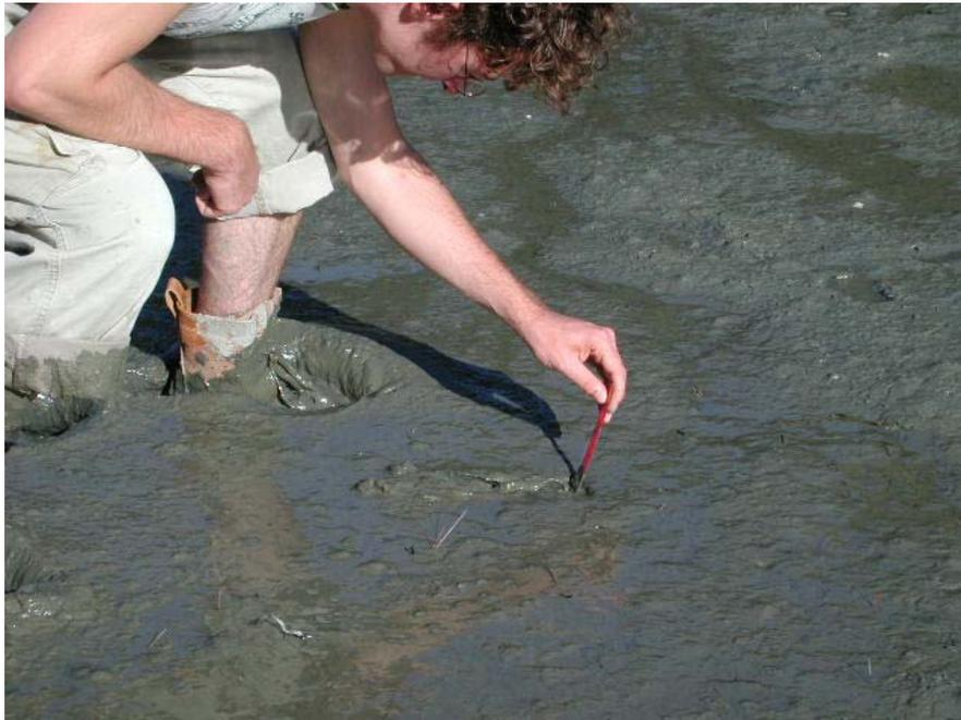
Figure 3. Measuring RPD depth.
